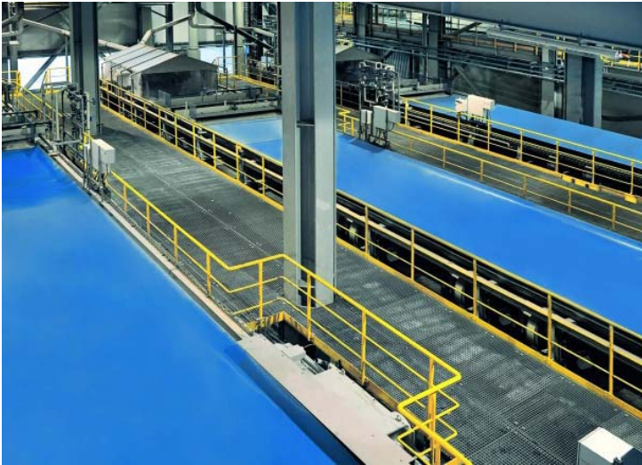
Picture 4: The VACUBELT® 2015 filter belt from GKD has been the globally established standard in the field of FGDP gypsum dewatering for many years.
